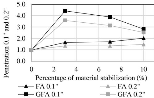
Fig. 9 CBR value of the stabilized soil
