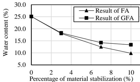
Fig. 2 Water content of the stabilized soil
