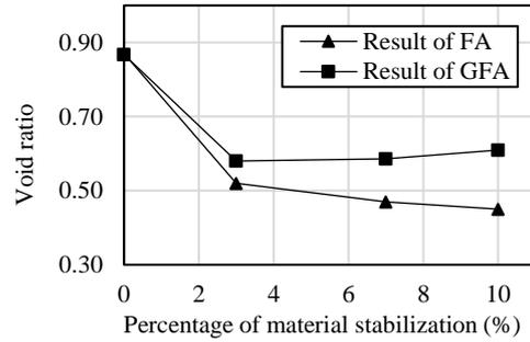
Fig. 4 Void ratio of the stabilized soil
