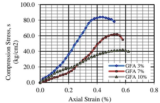
Fig. 7 Stress-strain relationship of the stabilized soil with geopolymer (GFA)
