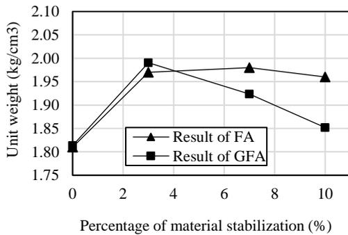
Fig. 3 Unit weight of the stabilized soil
