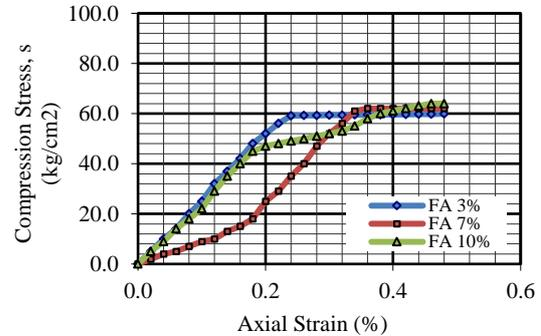
Fig. 6 Stress-strain relationship of the stabilized soil with fly ash (FA)
