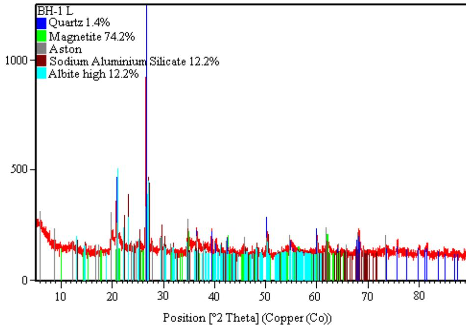
Fig. 1 XRD pattern of initial soil
