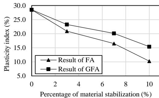
Fig. 5 Plasticity index of the stabilized soil
