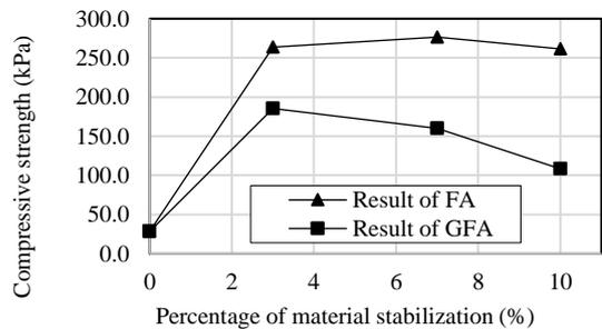
Fig. 8 Compressive strength of the stabilized soil
