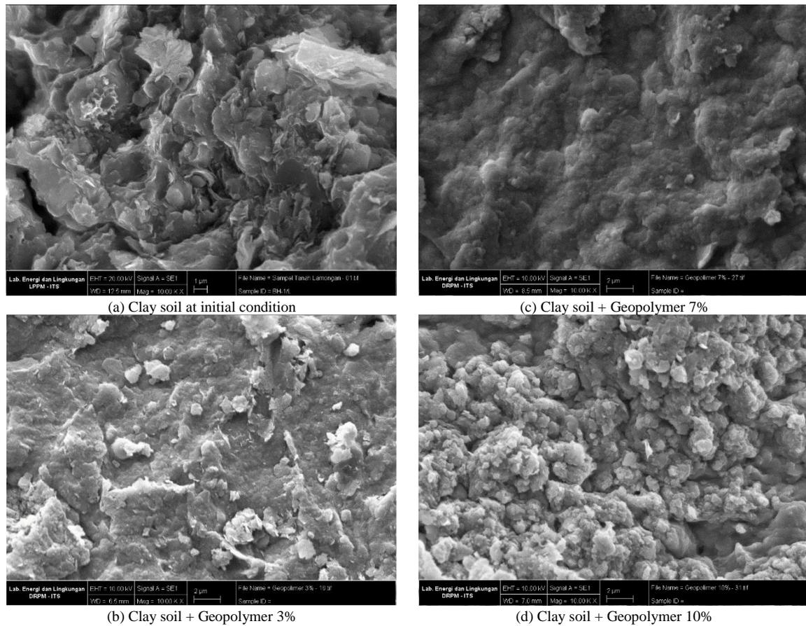
Fig. 11 Fig. 11 Micropores of clay (a) initial conditions (b) geopolymer stabilization 3% (c) geopolymer stabilization 7% (c) geopolymer stabilization 10%
