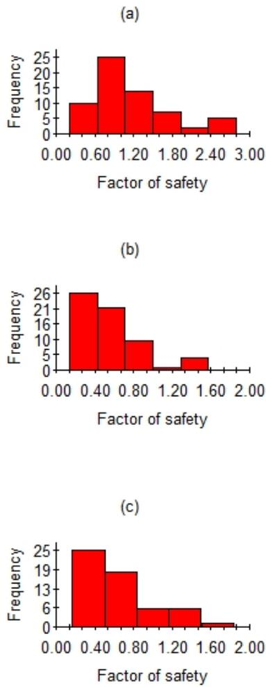
Fig.3 Histogram of the factor of safety (FS) against liquefaction for (a) 1m, (b) 3m and (c) 7m
