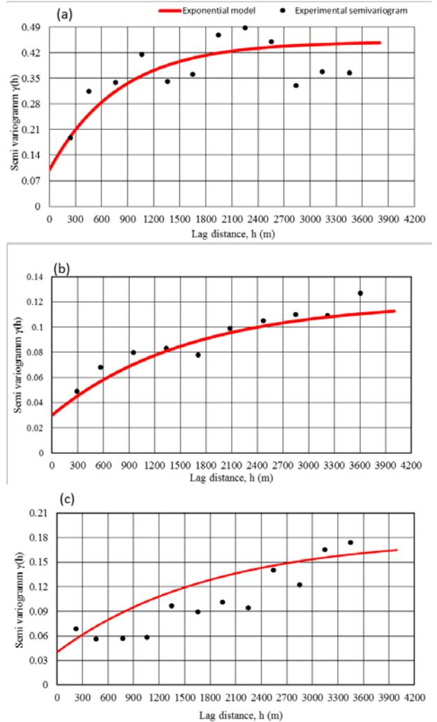
Fig.4 Experimental and theoretical semivariograms for FS (a) 1m, (b) 3m and (c) 7m
