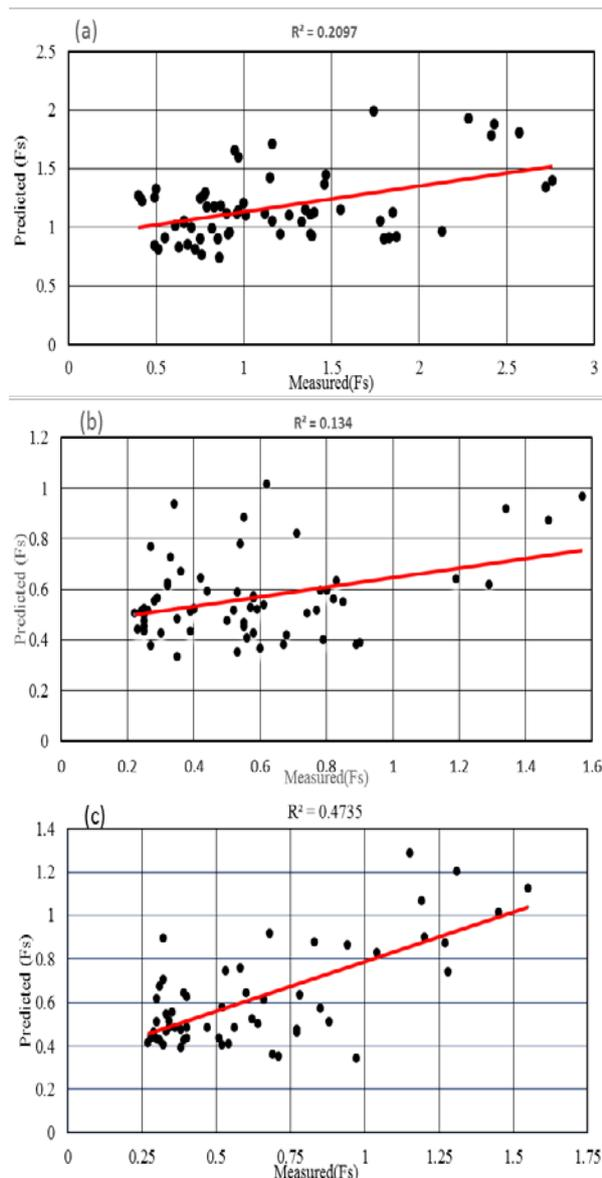
Fig.7 Cross validation of the semivariogram model for the factor of safety (FS (a) 1m, (b) 3m and (c) 7m)
