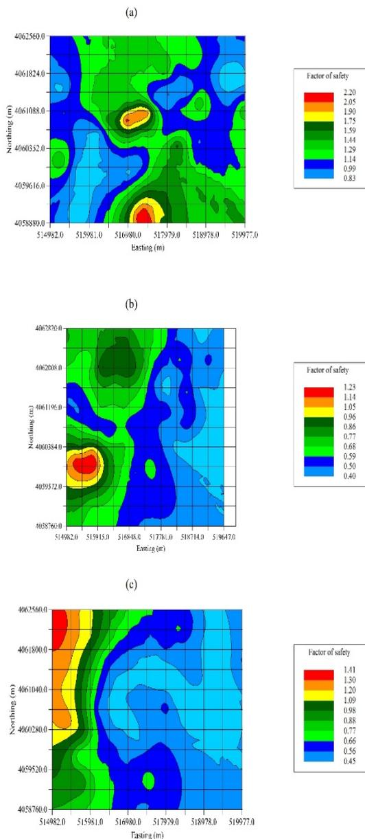
Fig.5 Factor of safety (FS (a) 1, (b) 3 and (c) 7m) hazard map predicted by ordinary kriging for
