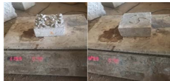
Fig. 8: Specimen's weight during sorptivity test.
