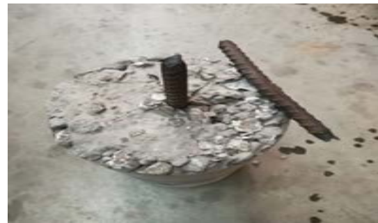
Fig. 7 b): Failure in the steel bar during pullout test.
