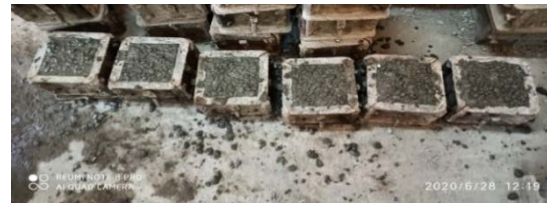
Fig. 3-c): Cube specimens for SCC – Mix 2
