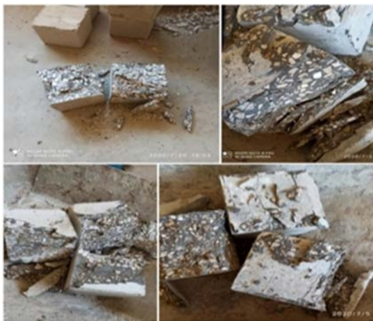
Fig. 6: failure mode of cubes
