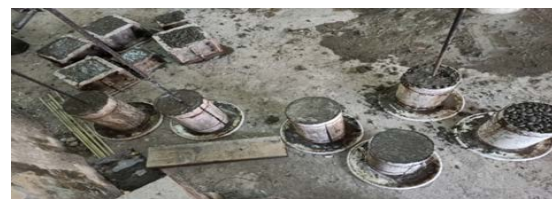
Fig. 4: Casting specimens for hardened tests without compaction.
