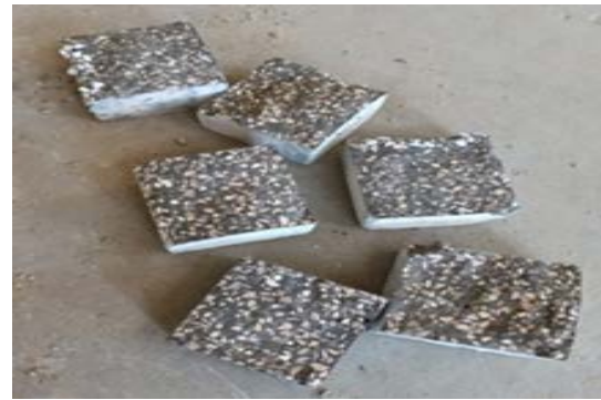
Fig. 7 a): Failure modes of cubes under splitting tensile test.
