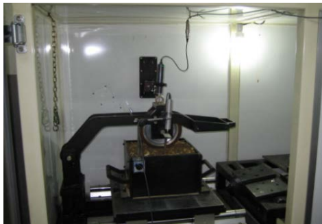
Fig.3 Wheel track load test
