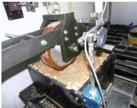
Fig.4 Measurer instruments of the settlement
