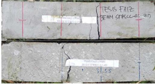
Fig.12 The specimen failure of the SFRSCC
