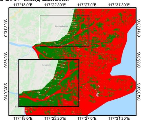
Fig. 6 Striping issues in Landsat 7 recording
