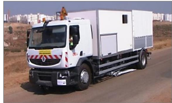
Fig.1 Lacroix Deflectograph measurement
