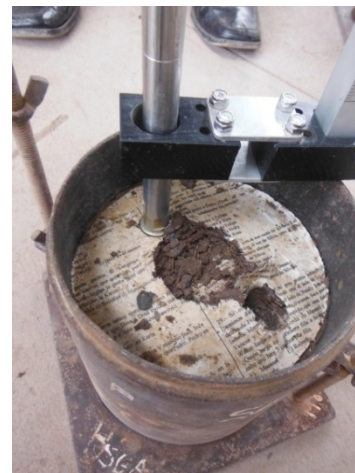
Fig.1 DCP perforation to one side of the CBR indentation.
