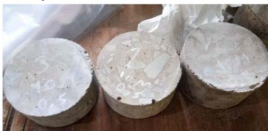
Fig. 5 Sample pieces for porosity test at 28 days old
