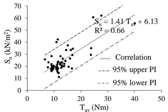
Fig. 6 Relationship between undrained shear strength ( $S_u$ ) from UU test and torque ( $T_{av}$ )
