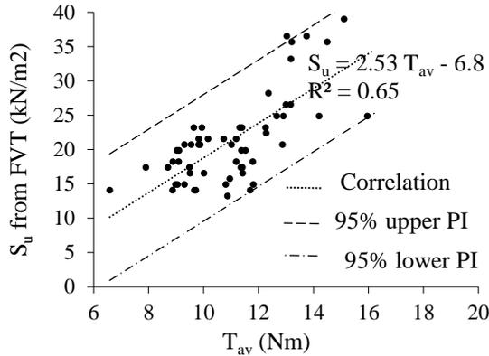
Fig. 7 Relationship between undisturbed undrained shear strength ( $S_u$ ) from FVT test and torque ( $T_{av}$ )
