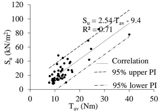
Fig. 5 Relationship between the undrained shear strength ( $S_u$ ) from UC test and torque ( $T_{av}$ )
