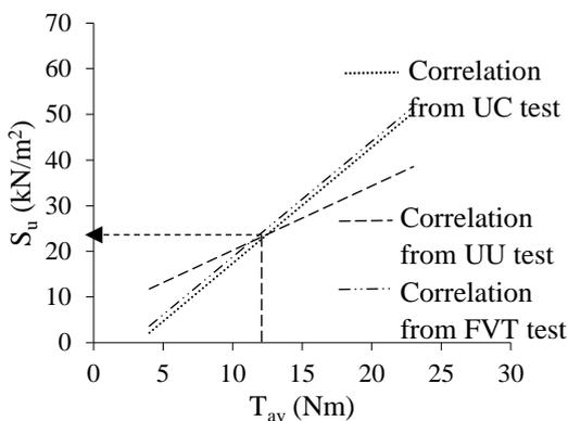
Fig. 8 Correlation between torque ( $T_{av}$ ) and undrained shear strength ( $S_u$ ) obtained from UC, UU, and FVT tests
