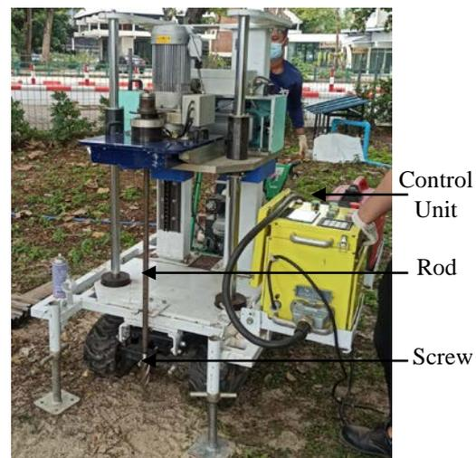
Fig. 2 Customized SDS equipment in action
