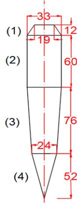
Fig. 4 SDS screw point depicted in simplified form, with dimensions in millimeters.
