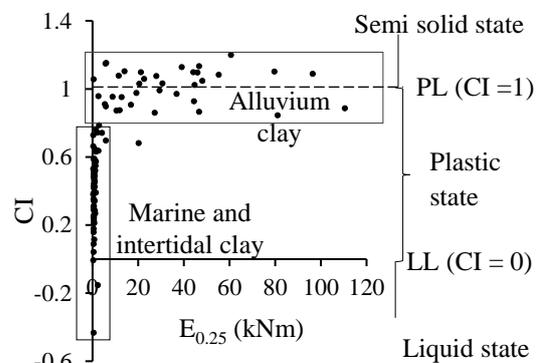
Fig. 10 Variation of penetration energy ( $E_{0.25}$ ) with consistency Index (CI)
