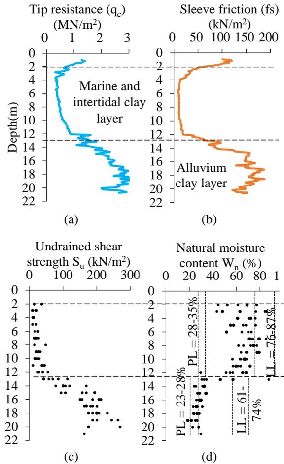
Fig. 3 a) Profile of CPT tip resistance ( $q_c$ ) on test site, b) Profile of CPT sleeve friction ( $f_s$ ) on test site, c) Profile of undrained shear strength ( $S_u$ ) with depth, d) Profile of natural moisture content on test site indicating liquid limit (LL) and plastic limit (PL) ranges of each type of soil layer
