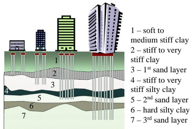
Fig. 1 Required depth of pile foundations during construction in Bangkok according to the type of super-structures [19]
