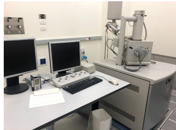
Fig. 2 Photograph of the scanning electron microscope (SEM) Inspects S50.
