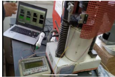
Fig. 3 Carrying out testing with the use of hydraulic measuring press PGI – 500.
