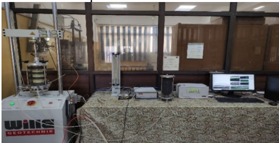
Fig. 4 The cyclic triaxial apparatus used in the study
