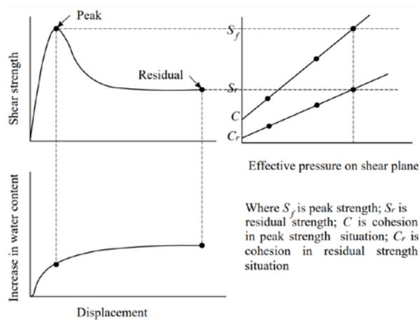
Fig. 1 Concept of residual strength in shear characteristics
