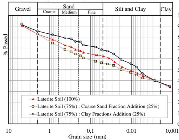
Fig. 3 Grain Size Distribution Curve
