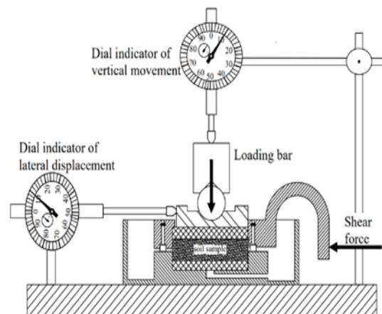
Fig. 2 Scheme for the Direct Shear Test Tool
