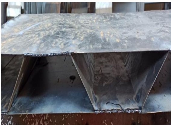
(c) Core web (middle corrugated plate and outer skins)
