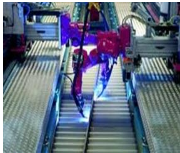
Fig.1 Automated production process of beams with corrugated webs [17]
