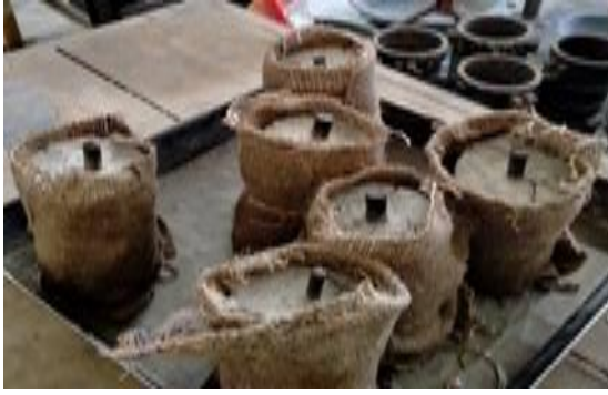
Fig.5b. Wrapped Specimens were sprinkled uniformly every day with water until the date of specimen testing.
