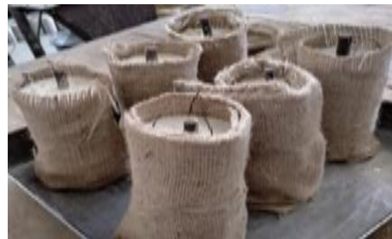
Fig.5a. Specimens were wrapped with Gunny Sack (burlap cover)
