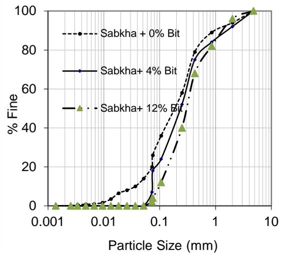
Fig.1: Grain size distribution curves for natural and bitumen mixed sabkha soil samples.
