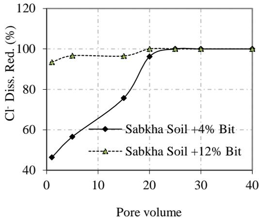
Fig.5 Chloride anion (Cl<sup>-</sup>) reduction rate vs. PV
