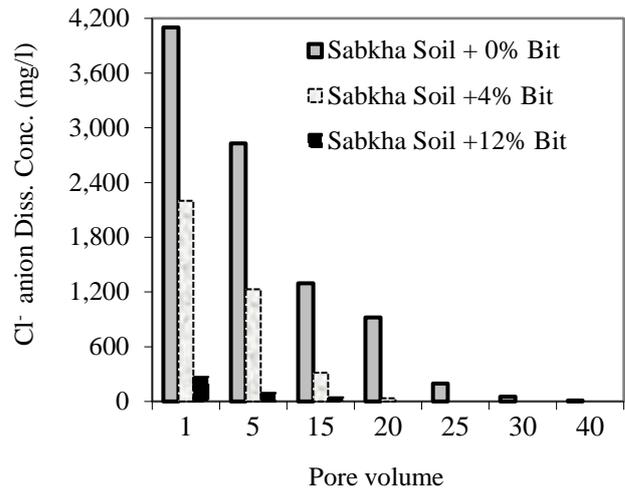
Fig.3 Chloride anion ( $\text{Cl}^-$ ) conc. vs. PV
