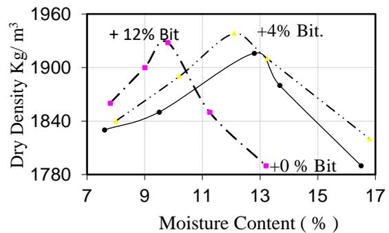
Fig.2 Dry density versus moisture content results
