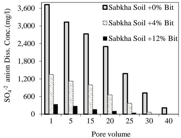
Fig.4 Sulfate anion ( $\text{SO}_4^{2-}$ ) conc. vs. PV
