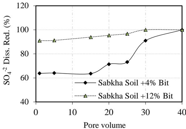
Fig.6 Sulfate anion (SO<sub>4</sub><sup>2-</sup>) reduction rate vs. PV
