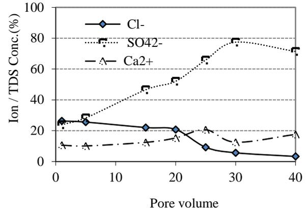
Fig.7 Main corrosive ion dissolution vs PV [1]
