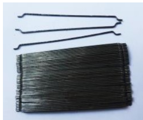
Fig.1 Steel fiber 3D, material properties: E=210,000 N/mm 2 , l=60 mm, d=0.75 mm, aspect ratio ( l/d )=80
