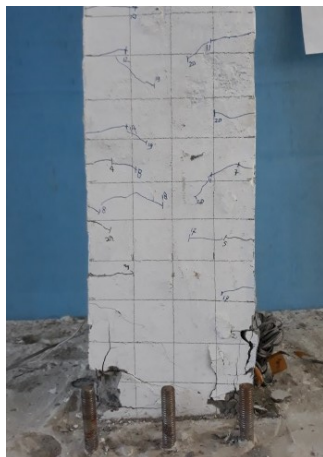
Fig.17 Column crack C_{50.2}
