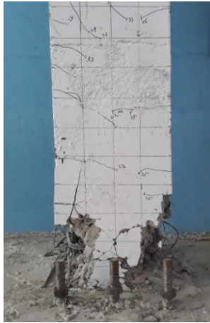
Fig.16 Column crack C_{50.1}
