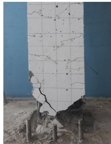
Fig.15 Column crack C 50.0
