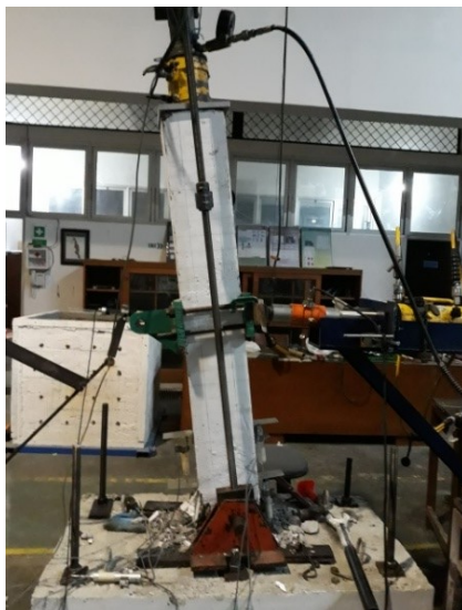
Fig.8 Collapsed condition of the column
