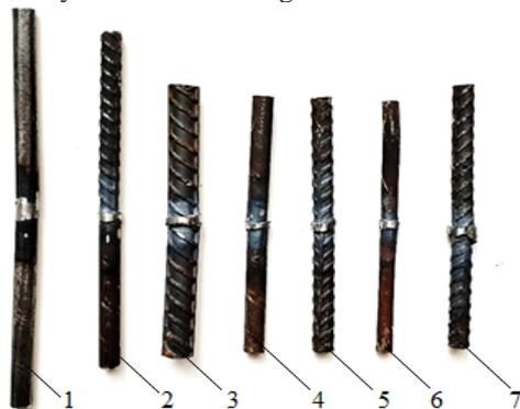
Fig.3 Samples of reinforcing bars joined by flash butt welding.
