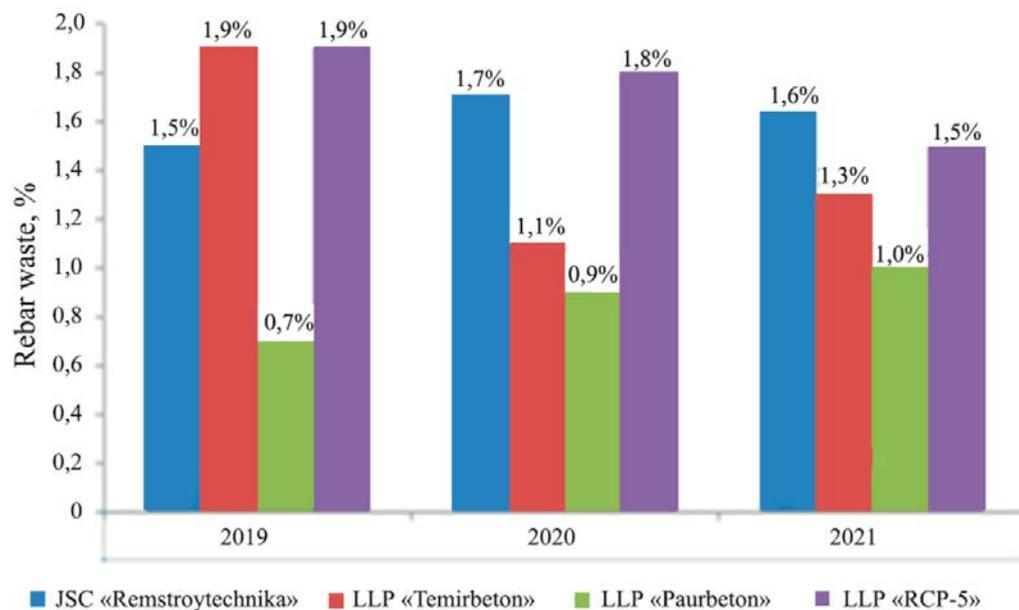
Fig.1 The percentage of waste reinforcing bars
