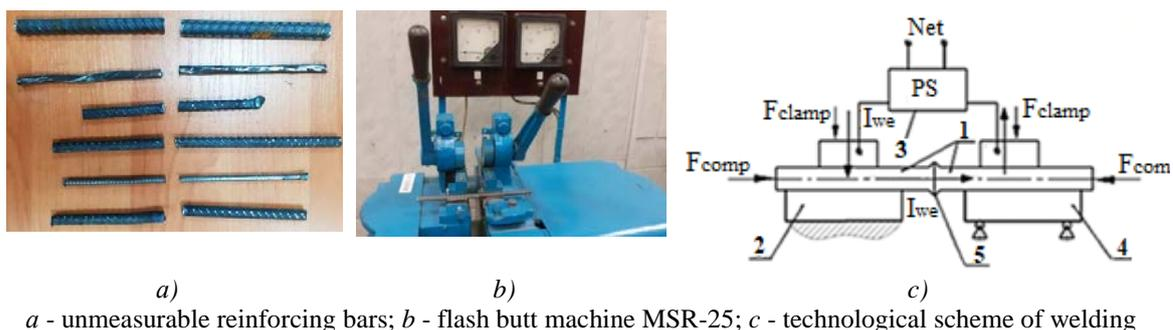
Fig.2 Unmeasurable reinforcing bars, flash butt machine MSR-25 and its technological scheme of welding
