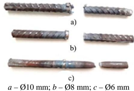
Fig.7 Some samples after tensile testing
