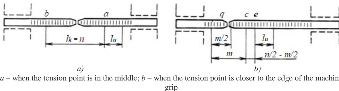
Fig.5 Schemes for determining the final calculated length of the sample
