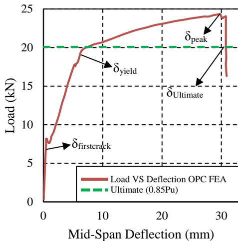
Fig. 10 Load-Deflection Curve of OPC Beam Structure using Finite Element Analysis
