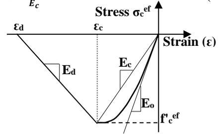
Fig. 4 Compressive Stress-Strain of Concrete Constitutive Model [31]
