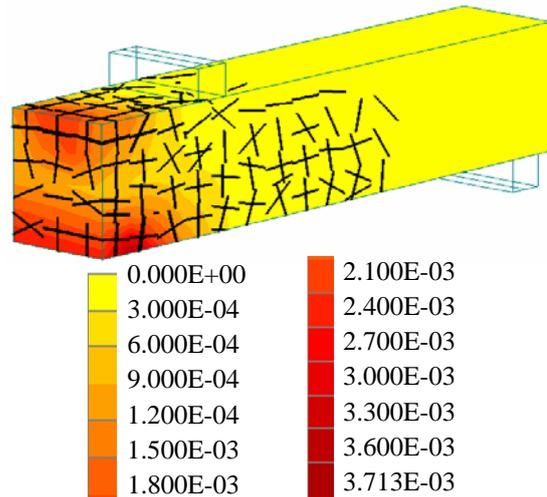
Fig. 14 Crack Pattern and Principal Strain OPC Beam Structure
