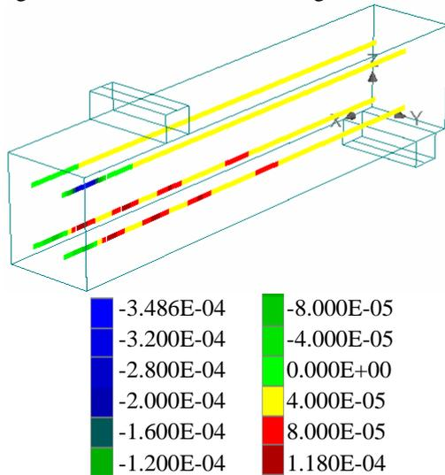
Fig. 9 Reinforcement Bond-Strength GPC Beam
