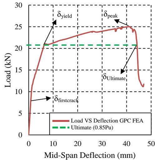
Fig. 11 Load-Deflection Curve of GPC Beam Structure using Finite Element Analysis
