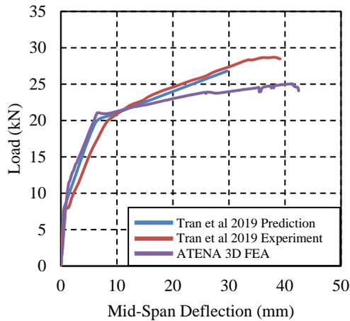
Fig. 13 Load – Deflection Curve Comparison GPC Beam Structure
