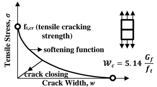
Fig. 5 Tension Stress-Strain of Concrete Constitutive Model [31],[32]
