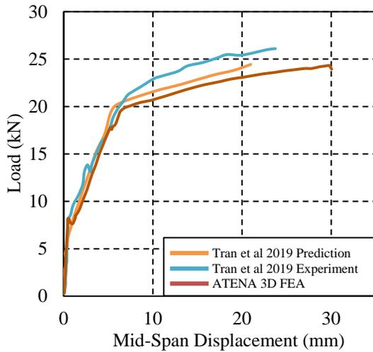
Fig. 12 Load – Deflection Curve Comparison OPC Beam Structure
