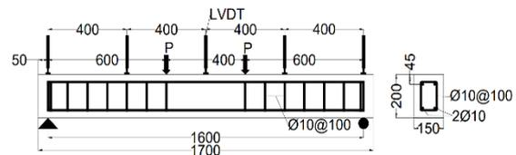
Fig. 1 Geometry and Cross Section of Beam Specimen [27]
