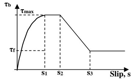
Fig. 7 Bond-Slip Law Based on CEB-FIP Model Code 1990 [31]
