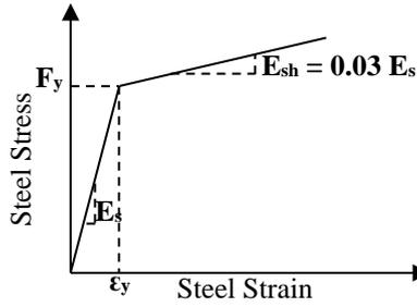
Fig. 6 Stress-Strain for Steel Reinforcement [27]
