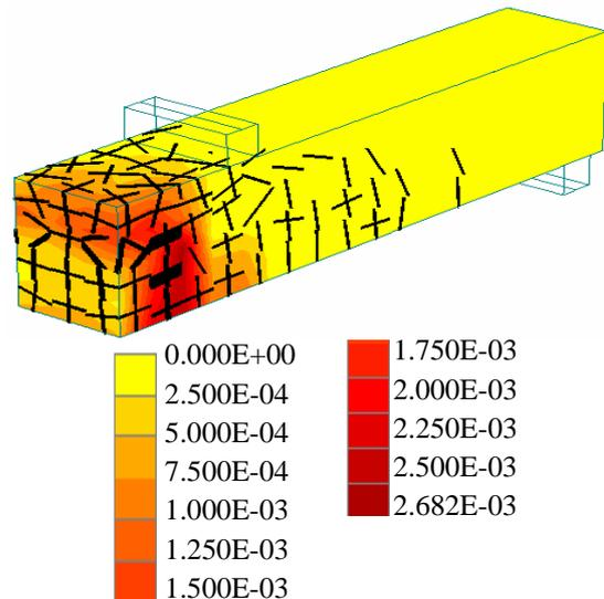
Fig. 15 Crack Pattern and Principal Strain GPC Beam Structure
