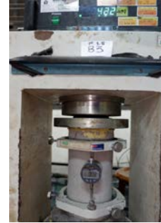
Fig. 1. Test model with the compressive test machine
