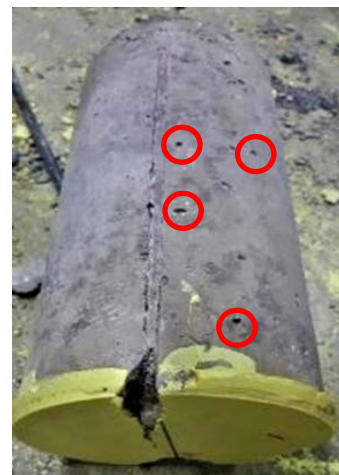
Fig. 4 Identified porous on the concrete surfaces.
