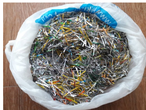
Fig. 2 Sample of fiber with a width of 2mm and length 40mm without interlocking shape.
