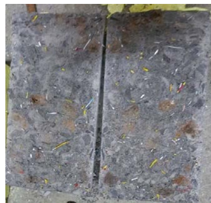
Fig. 12 Pumice distributions on the concrete with high fiber inclusions.
