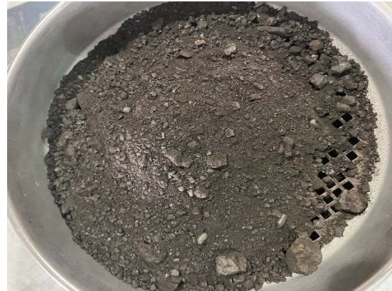
Fig.2 Screened CBA eliminates larger particles
