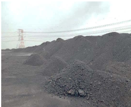
Fig.1 CBA produced by Manjung Power Plant in Perak
