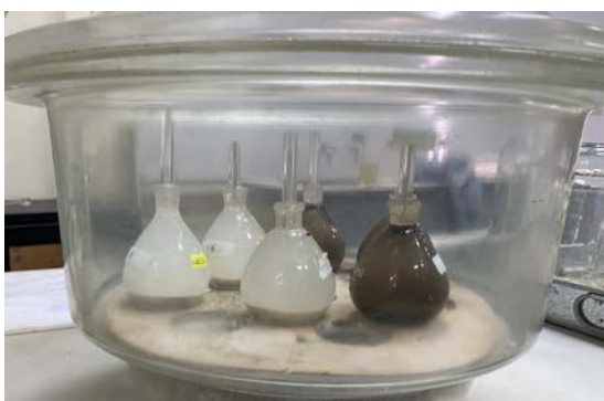
Fig.5 The pycnometer used to measure specific gravity of aggregates
