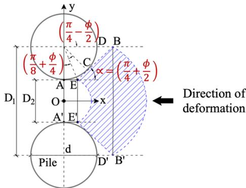
Fig. 1 Plastic deformation around the pile area [1]
