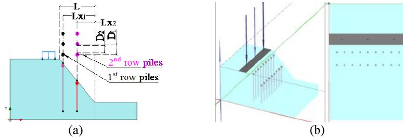
Fig. 3 The FEM slope modeling with two rows of piles: (a) 2D FEM and (b) 3D FEM
