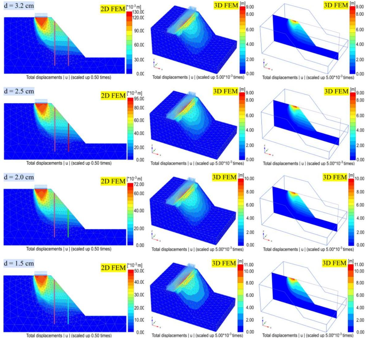
Fig. 10 Landslide zone of two-row pile reinforced slope
