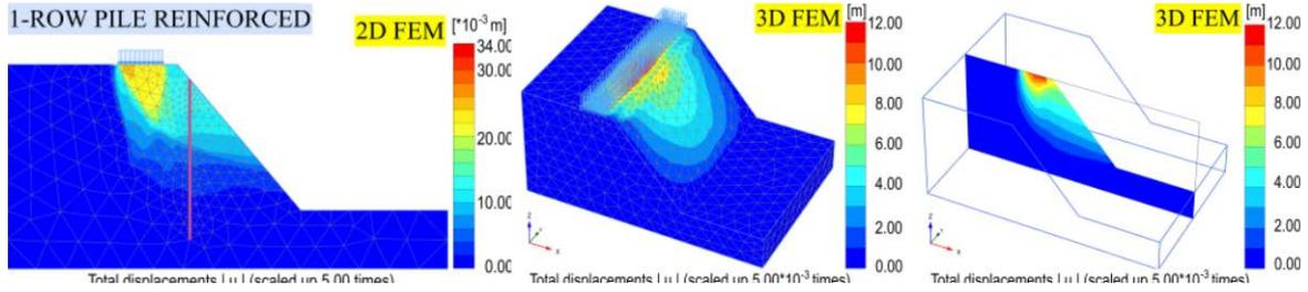
Fig. 9 Landslide zone of one-row pile reinforced slope
