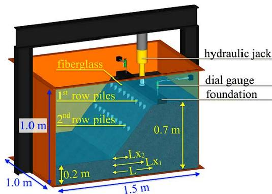
Fig. 2 The slope model configuration: (a) details of piles and (b) details of continuous footing
