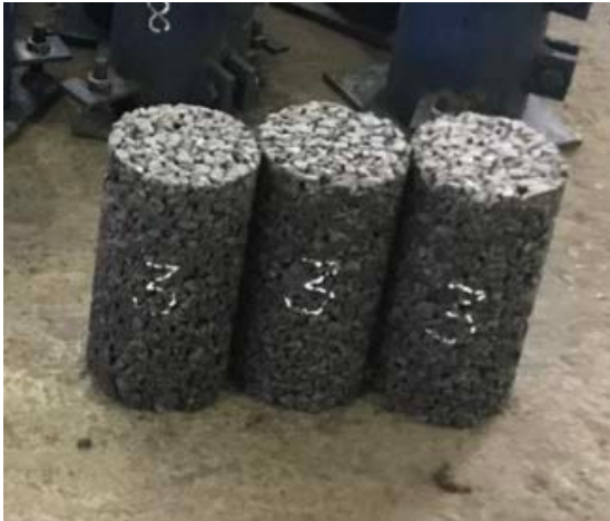
Fig. 2 Porous cement samples
