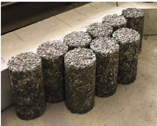
Fig. 3 Porous GPC samples
