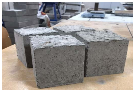
Fig. 1 Test samples—concrete cube samples
