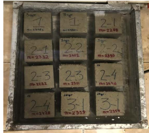
Fig. 4 Water saturation tests
