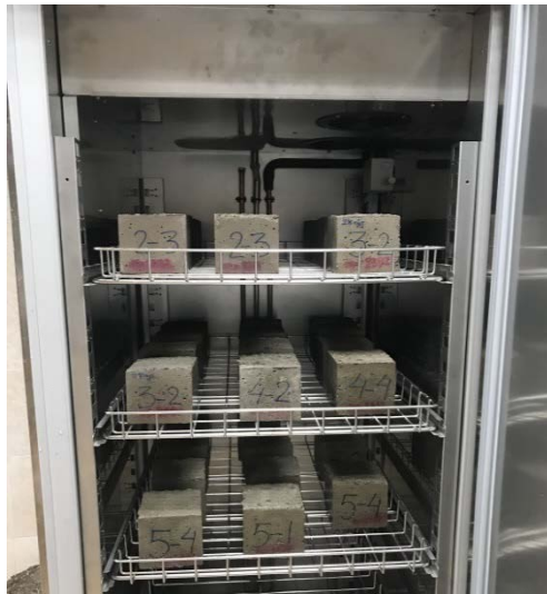
Fig. 3 Frost resistance tests
