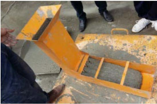
Fig. 3. The design of the L-shaped box and an example of its use in practice
