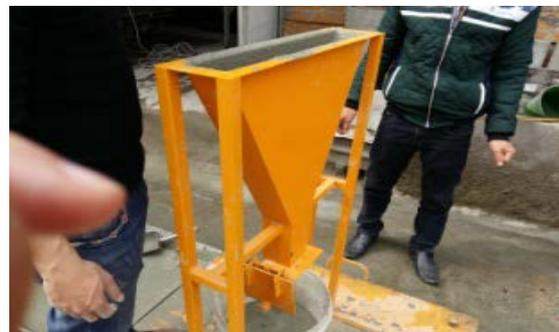
Fig. 2. The design of the V-shaped funnel and an example of its use in practical [5]
