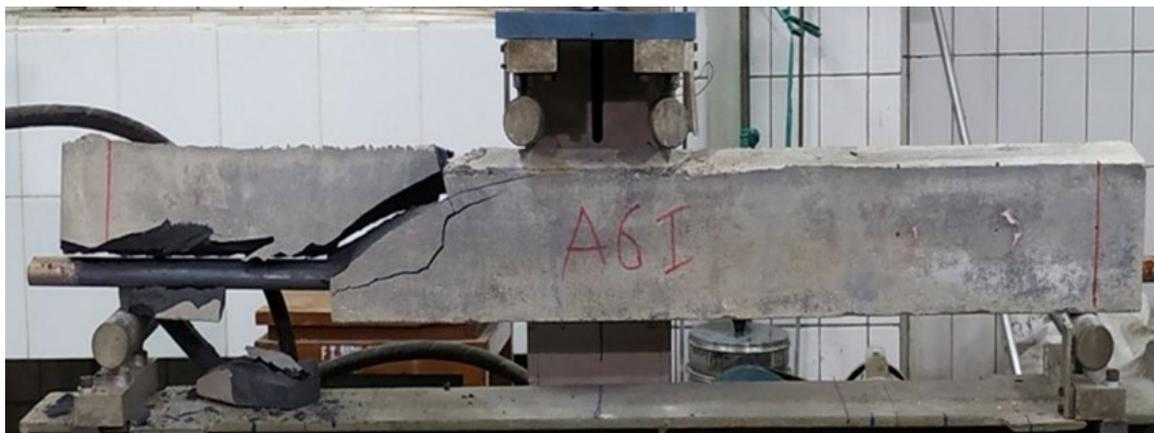
Fig.12 Beam A61 undergoes shear failure
