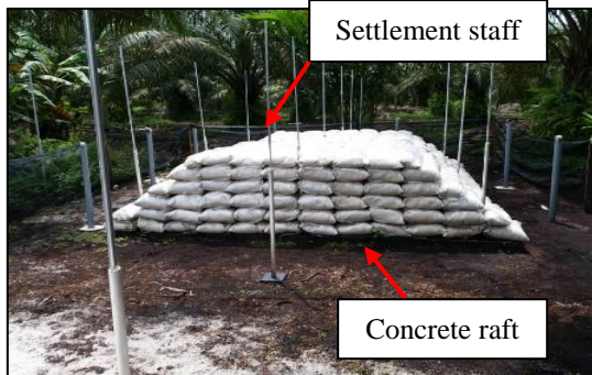
Fig. 2 Setting up of raft for non-uniform loading
