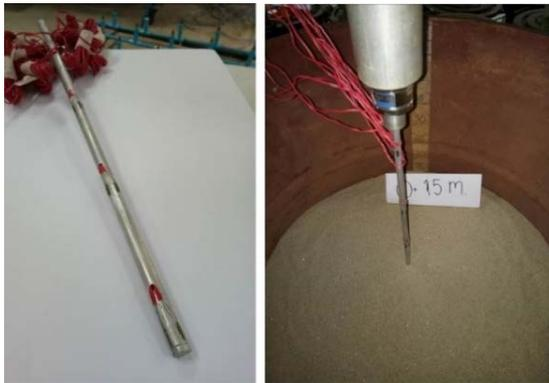
Fig.8 Hollow aluminium pile with cable strain gauges inside the pile
