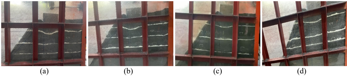
Fig. 3 The small-scaled model failure zone with the double-row pile, (a) D_1=5d ; (b) D_1=4d ; (c) 3d ; (d) D_1=2d
