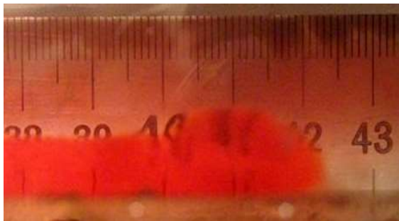
Fig.7 (a) The side snapshot of the head of the gravity current in the case of 1% density difference in bottom friction case.
