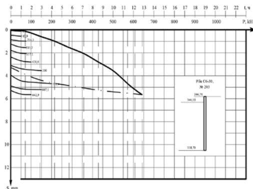
Fig.3 Correlation between settlement S and load P, the results of field static test on pile293
