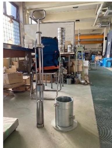
Fig. 2 Proctor Test Apparatus used to calculate the density of SMSW
