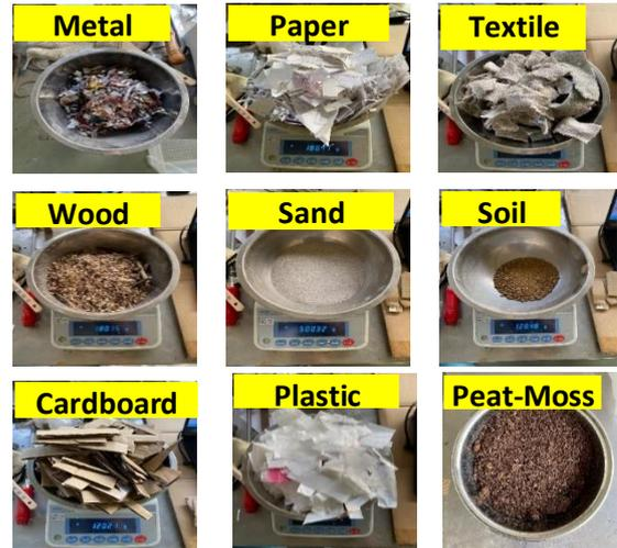
Fig. 1 Material Used in the Present study to build the synthetic waste
