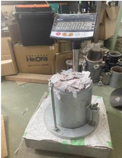
Fig. 3 Sample weighing after Compaction
