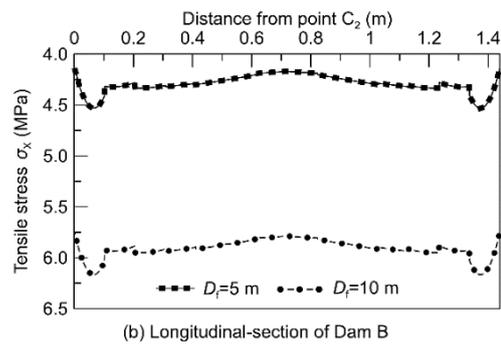
Fig. 13 Effect of depth of foundation on tensile stress  $\sigma_x$  of box culvert along  $C_2D_2$  ( $E_f=2$  MPa,  $E_c=21$  GPa)
