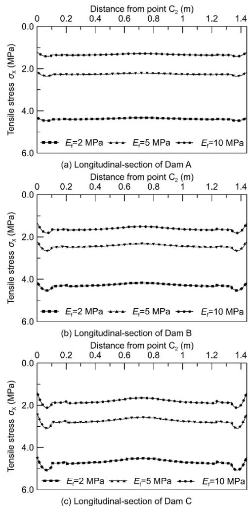
Fig. 9 Distribution of tensile stress  $\sigma_x$  of box culvert along  $C_2D_2$  ( $D_f = 5$  m,  $E_c = 21$  GPa)
