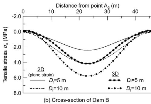
Fig. 12 Effect of depth of foundation on tensile stress  $\sigma_x$  of box culvert along  $A_2B_2$  ( $E_f=2$  MPa,  $E_c=21$  GPa)
