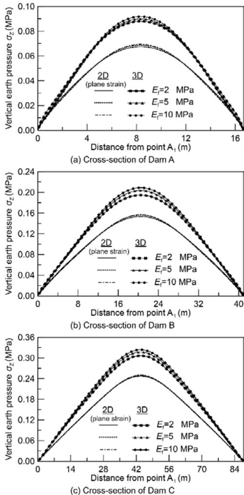
Fig. 6 Distribution of vertical earth pressure along  $A_1B_1$  ( $D_f = 5$  m,  $E_c = 21$  GPa)
