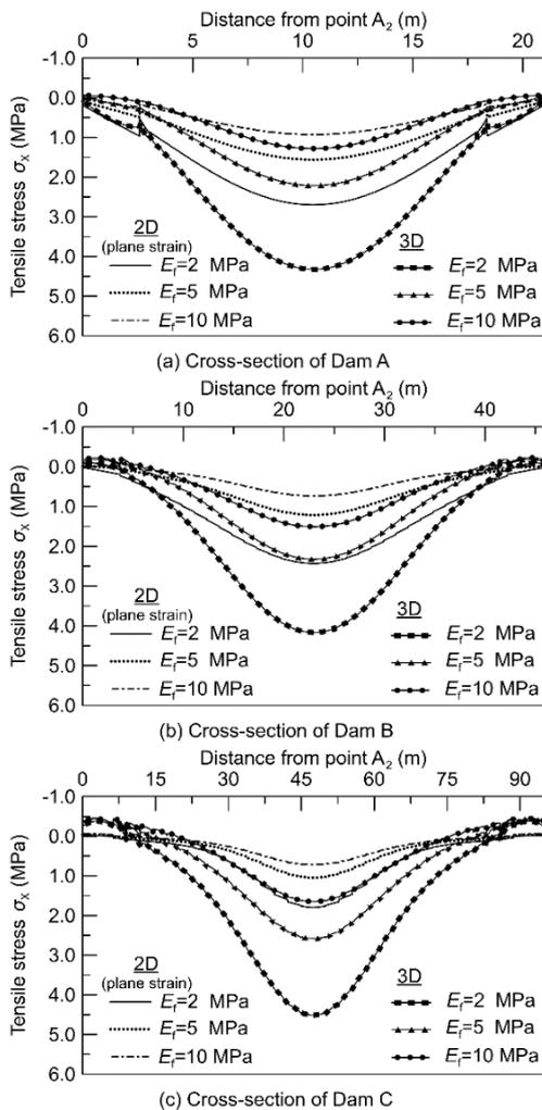
Fig. 8 Distribution of tensile stress  $\sigma_x$  of box culvert along  $A_2B_2$  ( $D_f = 5$  m,  $E_c = 21$  GPa)
