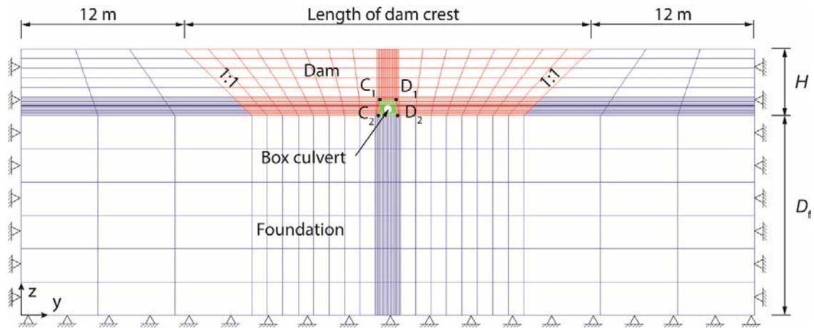
Fig. 4 Finite element mesh for dam longitudinal-section (2D plane stress FEM)
