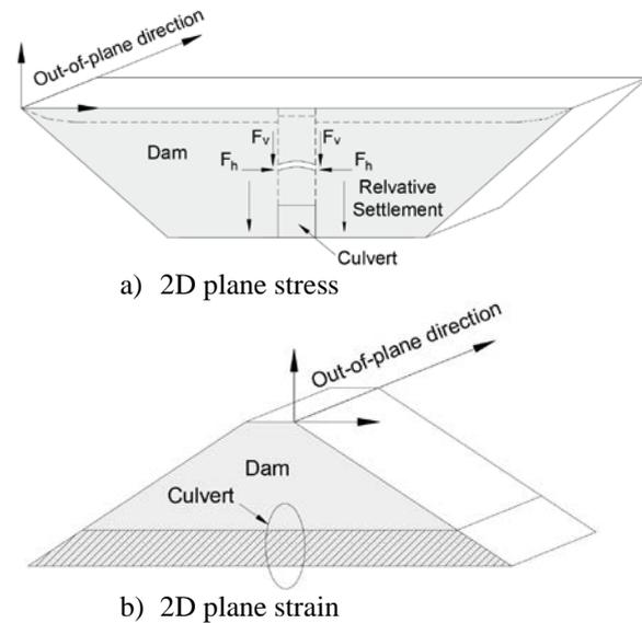
Fig. 1 2D (plane strain, plane stress) modeling for dam-culvert system
