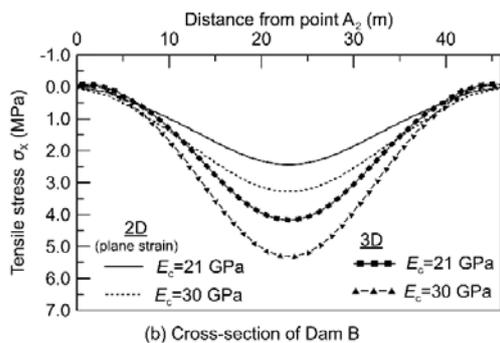
Fig. 10 Effect of stiffness of culvert on tensile stress  $\sigma_x$  of box culvert along  $A_2B_2$  ( $D_f = 5$  m,  $E_f = 2$  MPa)
