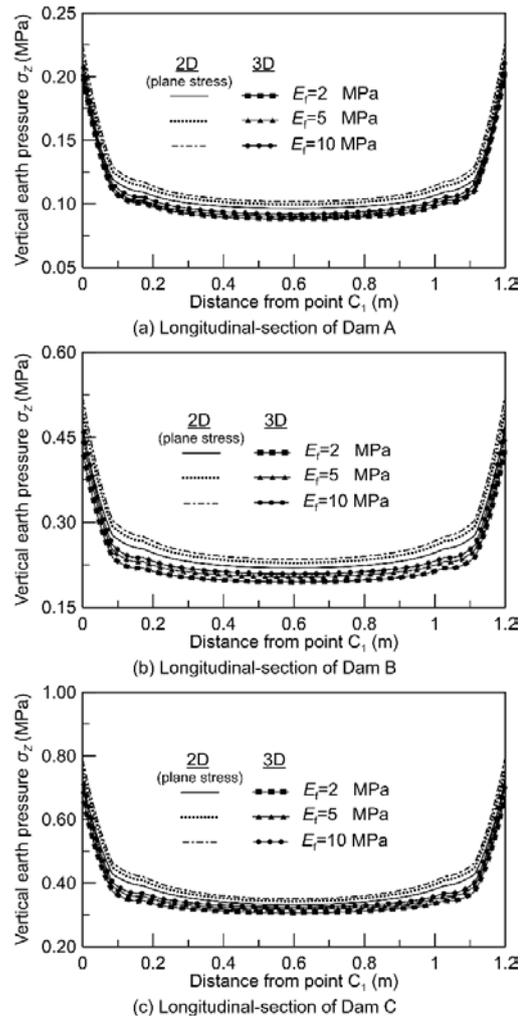
Fig. 7 Distribution of vertical earth pressure along  $C_1D_1$  ( $D_f = 5$  m,  $E_c = 21$  GPa)
