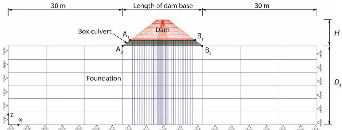
Fig. 3 Finite element mesh for dam cross-section (2D plane strain FEM)
