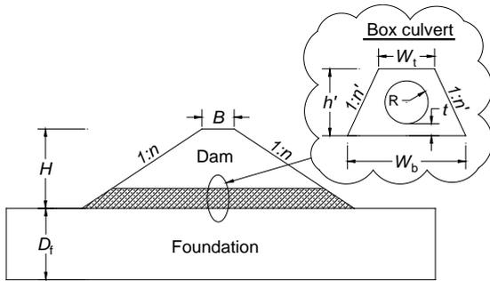
Fig. 2 Schematic illustration of typical dam-culvert-foundation system
