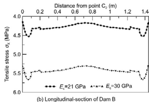
Fig. 11 Effect of stiffness of culvert on tensile stress  $\sigma_x$  of box culvert along  $C_2D_2$  ( $D_f = 5$  m,  $E_f = 2$  MPa)
