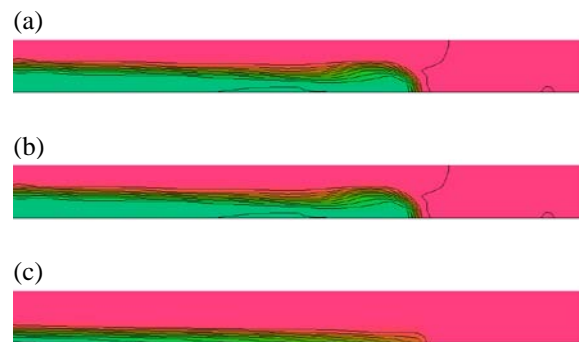
Fig.8 Contour maps of density of gravity currents at (a) t/T=20 , (b) t/T=80 , and (c) t/T=200 ( Re=1116 )
