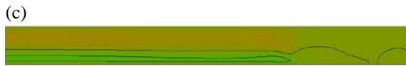
Fig.9 Contour maps of horizontal velocity of gravity currents at (a) t/T=20 , (b) t/T=80 , and (c) t/T=200 ( Re=1116 )
