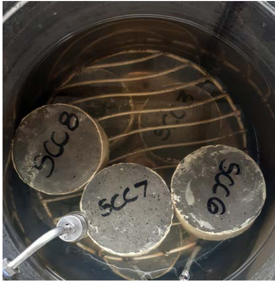
Fig. 1 Preparation of Samples for RCPT
