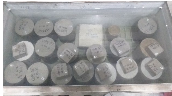
Fig. 6 The curing of specimens
