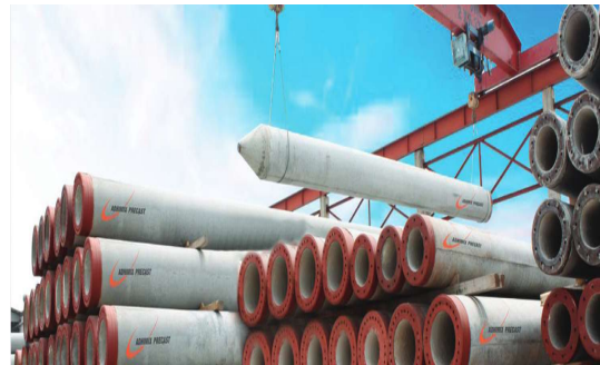
Fig. 1 Precast Product Spunpile
