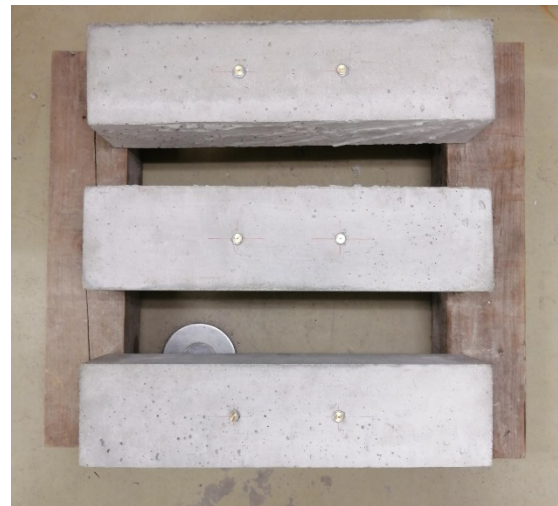
Fig. 3 The specimen after contact chips were attached
