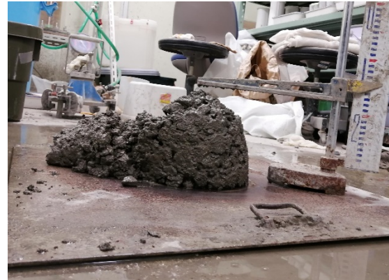
Fig. 5 Shape of WBA concrete
