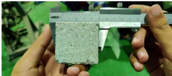
Fig. 5 Concrete blocks for physical properties testing.
