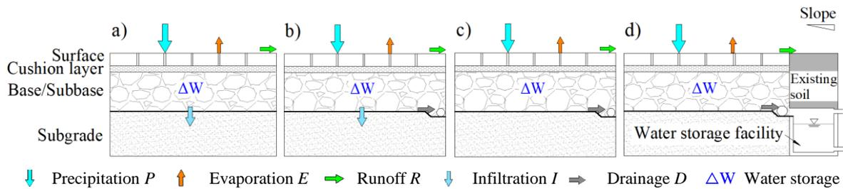
Fig. 2 Typical structure and components of water balance (modified after [3,6,39-41]) for a) full infiltration, b) partial infiltration, c) no infiltration, and d) no infiltration with a water storage facility
