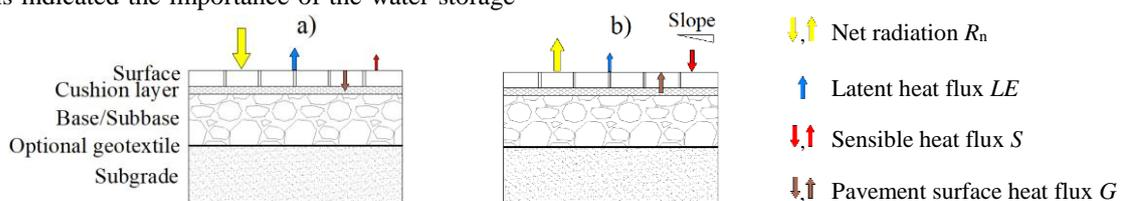
Fig. 3 Typical components of the surface heat flux balance (modified after [14,19]) for a) daytime, and b) nighttime
