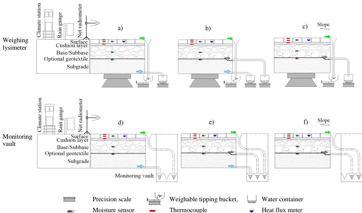
Fig. 4 Schematic of a monitoring system for measuring water (modified after [33,39-41,47]) and heat (modified after [14,19]) balance components using weighing lysimeter and monitoring vault system for a, d) full infiltration; b, e) partial infiltration, and c, f) no infiltration type
