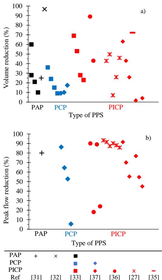
Fig. 1 The effect of type of PPS on a) volume reduction, b) peak flow reduction
