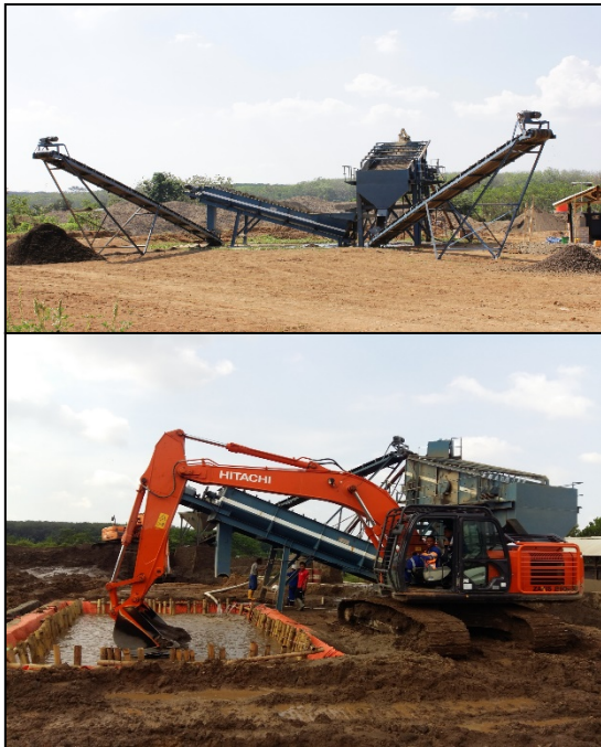
Fig. 5 The sand production process uses a vibrating screen machine (upper photo) and a sand-washing pond (lower photo).
