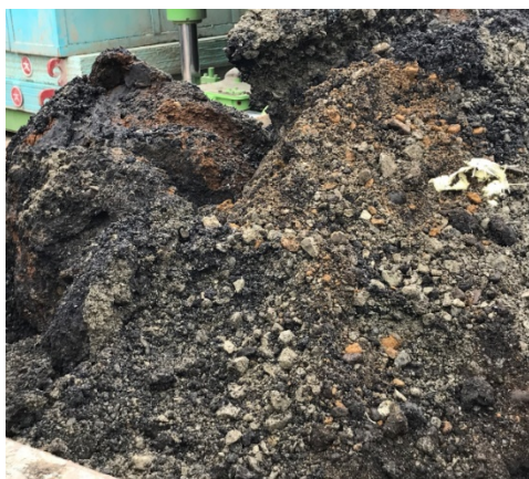
Photo 1 Excavated Coal cinders from redevelopment project in the railroad site
