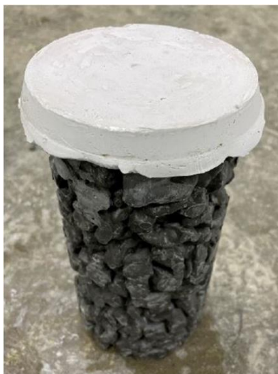
Fig. 2 The specimen on which the upper end surface is covered with gypsum
