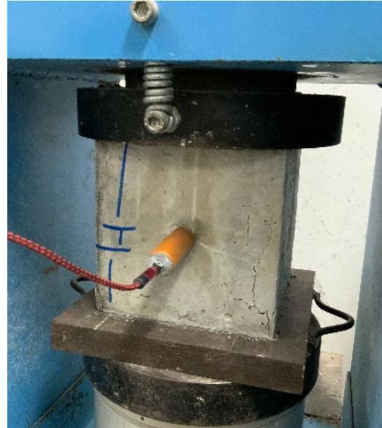
Fig. 6 Installed Sensor to Measure Magnitude (Volt<sup>2</sup>) in Concrete Samples
