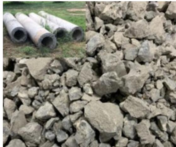
Fig. 1 Recycled Aggregates from Pile Waste
