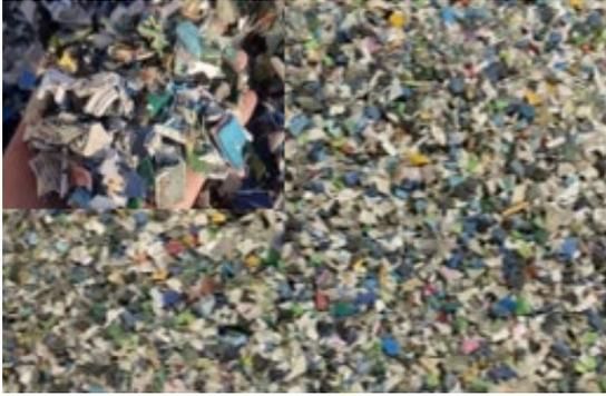
Fig. 3 Plastic Waste Used as a Replacement for Fine Aggregate in Concrete Mixes
