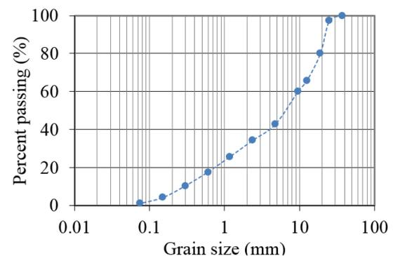
Fig. 2 Gradation Curve of Recycled Aggregates
