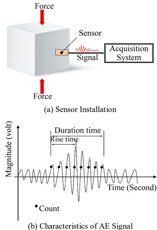
Fig. 5 Sensor Installation and Characteristics of AE Signal
