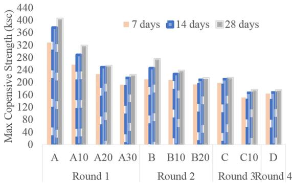
Fig. 8 Comparison of Maximum Compressive Strength of Recycled Concrete after 7, 14, and 28 Days of Water Curing in Each Recycling Cycle
