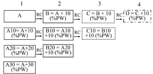
Fig. 4 Flow Chart of Recycled Concrete Sample Preparation
