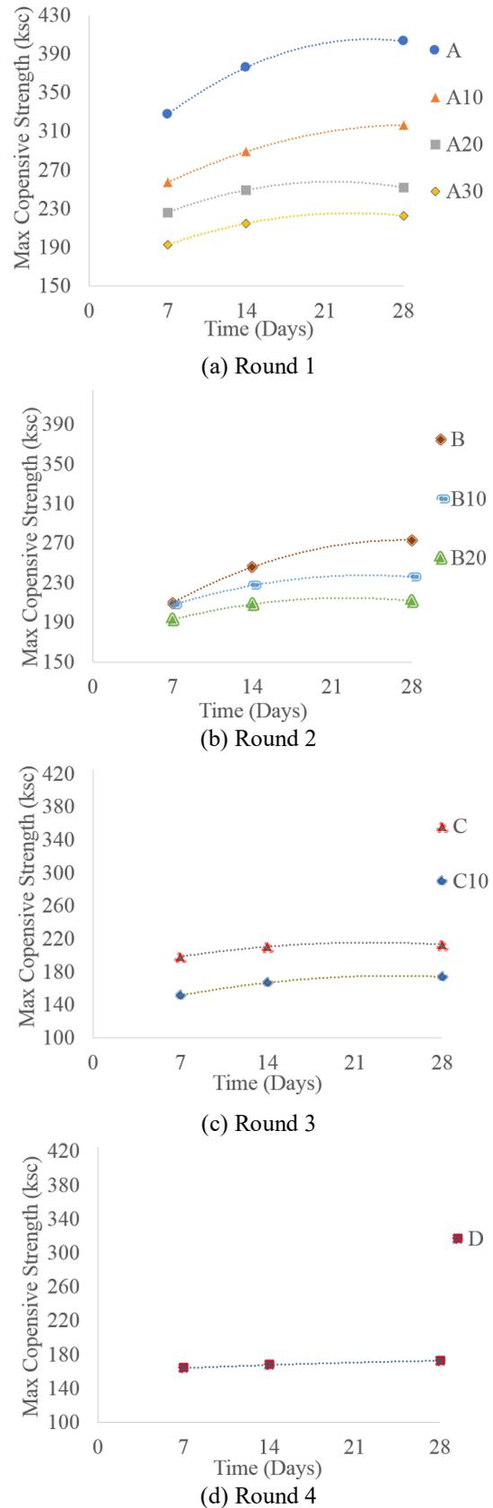
Fig. 7 Maximum Compressive Strength of Recycled Concrete after 7, 14, and 28 Days of Water Curing
