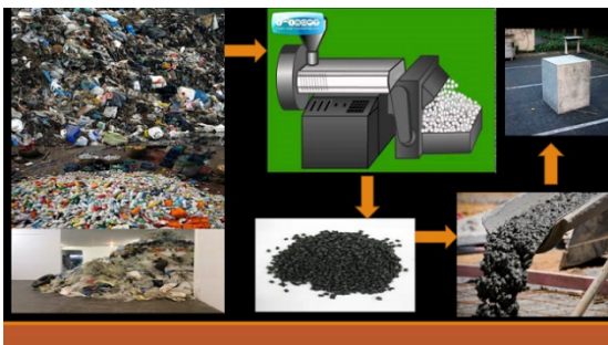
Fig. 4 Plastic granules manufacture process
