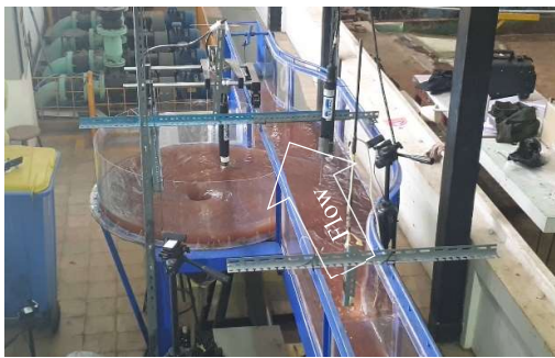
Fig. 9 Flushed removal out of sediment's fraction
