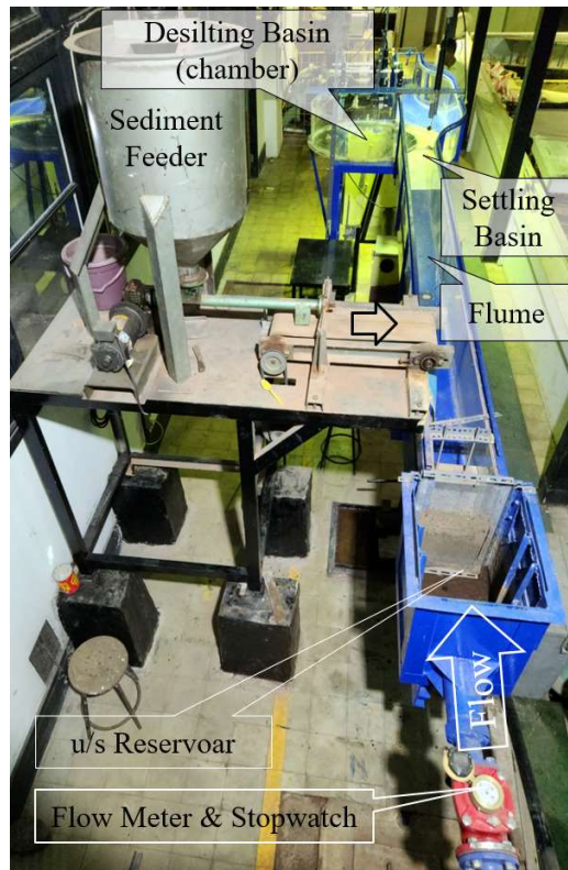
Fig. 4 Visual view of the laboratory test undistorted physical model with a scale of 1:40
