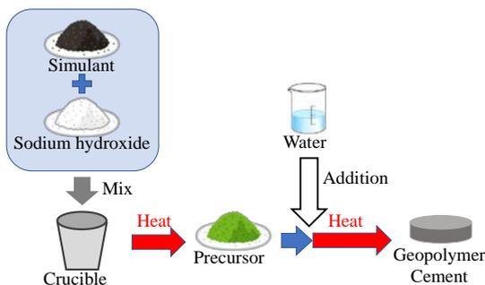
Fig.1 Geopolymer cement preparation method
