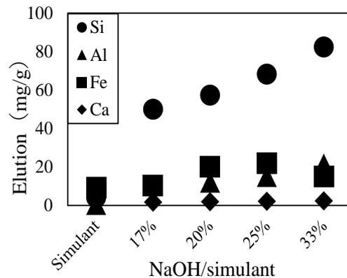
Fig.8 Elution of Si, Al, Fe and Ca from precursor of geopolymer with various NaOH addition
