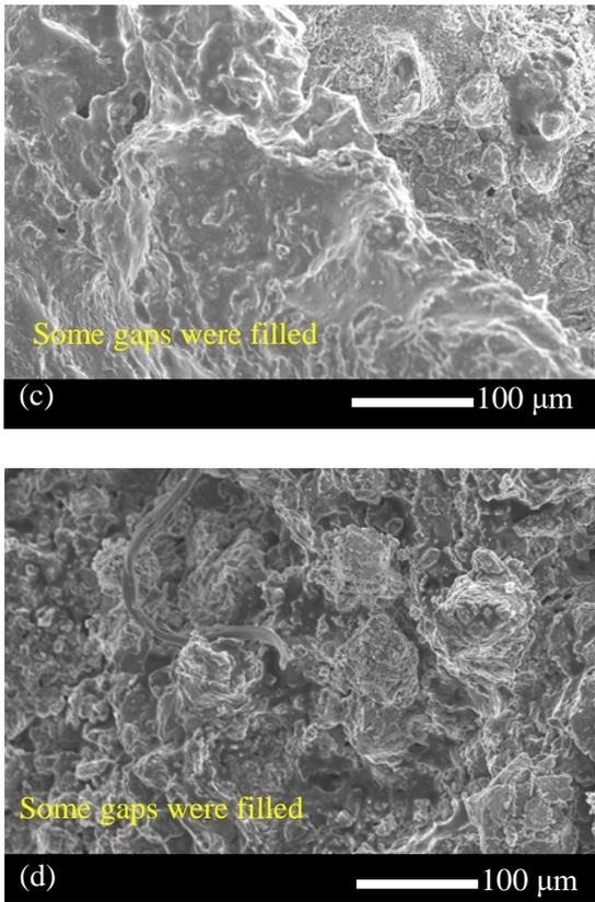
Fig.12 SEM photos for cross sections of products prepared by heating at (a)1 h, (b)1.5 h, (c)2 h, and (d)3 h
