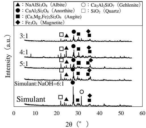
Fig.5 XRD patterns of the geopolymer cements prepared with different ratios of sodium hydroxide
