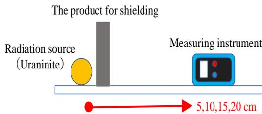
Fig.4 Radiation shielding measurement method
