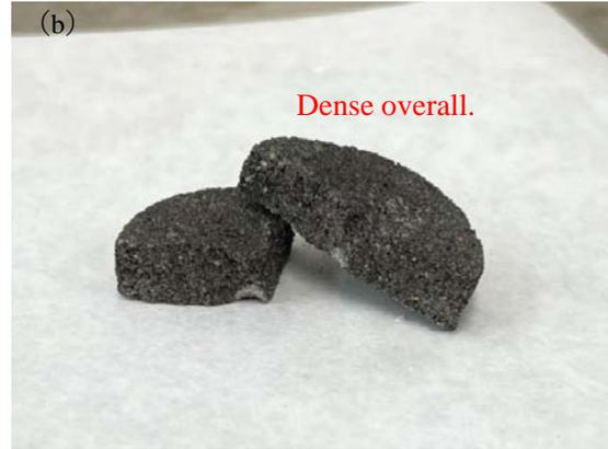
Fig.7 The cross section of samples after strength test; (a) water ratios greater than 25% and (b) water ratios less than 25%
