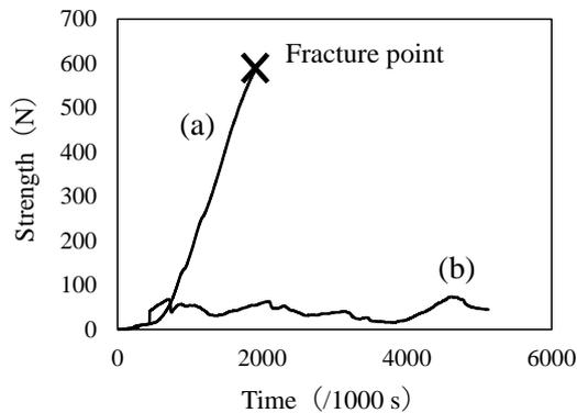
Fig.6 The strength of typical geopolymer cements among the prepared samples; (a) sample with low water content and (b) sample with high water content
