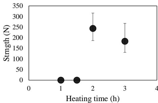
Fig.10 The maximum breaking load of the prepared geopolymer cement as a function of heating time
