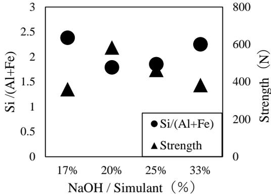
Fig.9 Ratio of the amount of metals dissolved from the precursor of geopolymer with various NaOH addition and the strength of their prepared products
