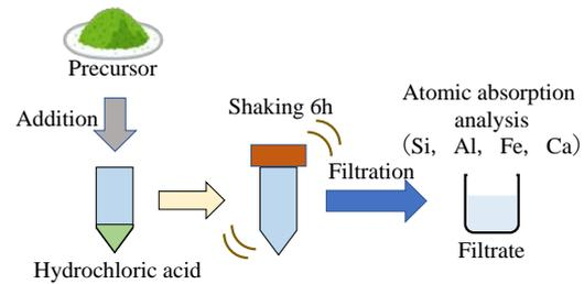
Fig.2 Metal elution measurement method
