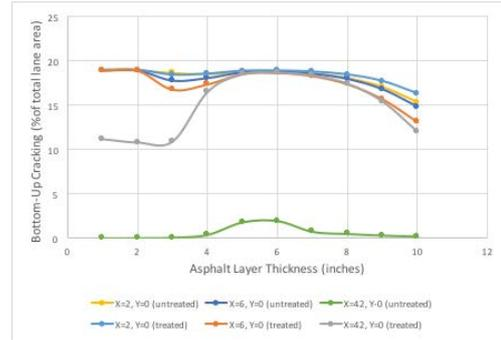
Fig.15 Result for bottom-up cracking at the most critical and least critical locations for rural roads
