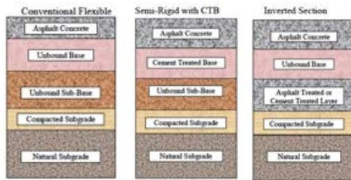
Fig.1 Possible asphalt layered systems [7]
