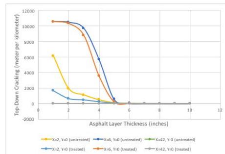
Fig.12 Result for top-down cracking at the most critical and least critical locations for urban roads
