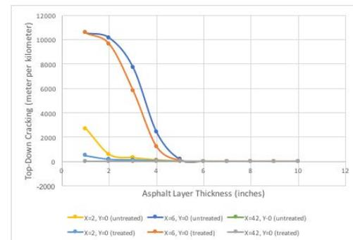
Fig.16 Result for top-down cracking at the most critical and least critical locations for rural roads
