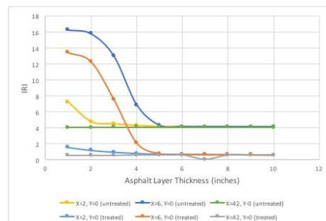
Fig.18 Result for IRI at the most critical and least critical locations for rural roads
