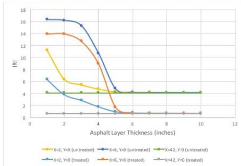
Fig.14 Result for IRI at the most critical and least critical locations for urban roads
