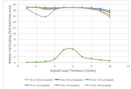
Fig.11 Result for bottom-up cracking at the most critical and least critical locations for urban roads
