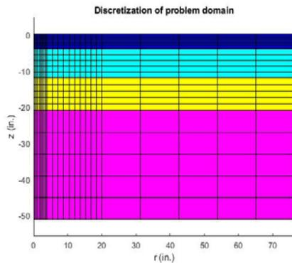
Fig. 6 Sample pavement model with discretization
