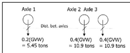
Fig.2 Load distribution for each 3-axle [11]
