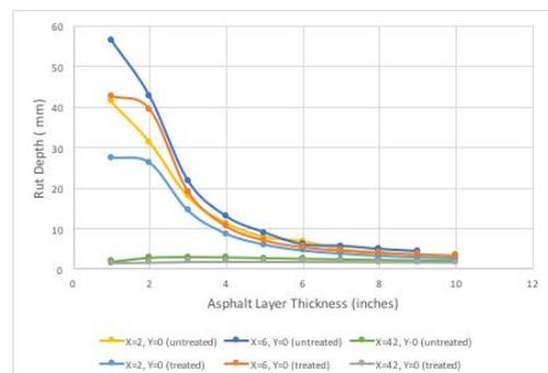
Fig.17 Result for rut depth at the most critical and least critical locations for rural roads
