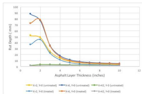
Fig.9 Result for rut depth at the most critical and least critical locations for heavily trafficked roads
