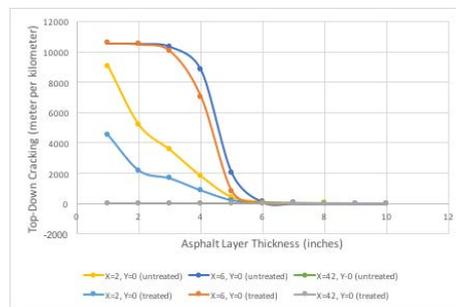
Fig.8 Result for top-down cracking at the most critical and least critical locations for heavily trafficked roads
