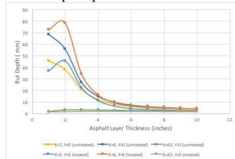
Fig.13 Result for rut depth at the most critical and least critical locations for urban roads
