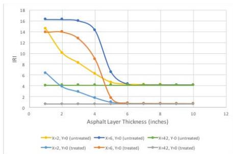
Fig.10 Result for IRI at the most critical and least critical locations for heavily trafficked roads
