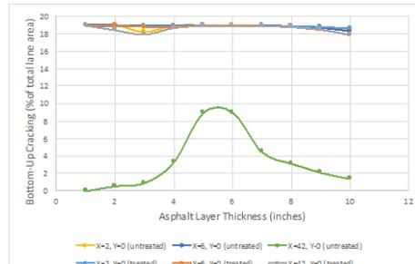
Fig.7 Result for bottom-up cracking at the most critical and least critical locations for heavily trafficked roads
