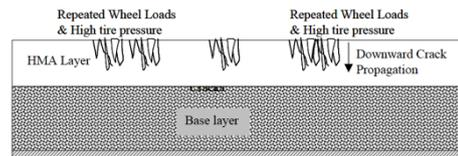
Fig. 5 Surface-down Fatigue Cracking
